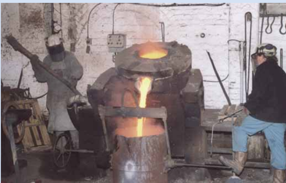
Removing the molten metal from the furnace prior to casting.
