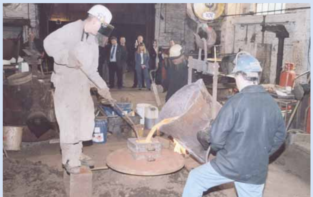
Casting the bell, the metal is an alloy of copper and tin.
